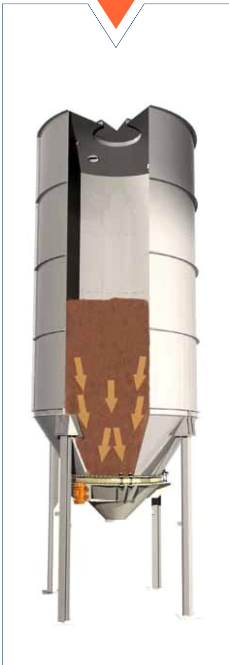
Ratholing Bridging Segregation Incomplete emptying
